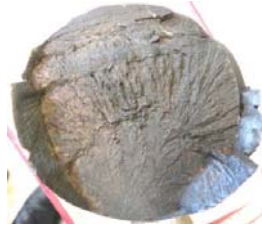
Rupture brutale semi-fragile
