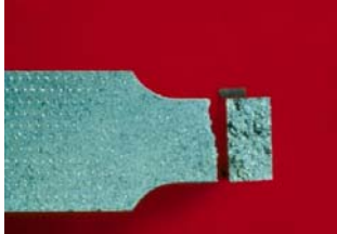
Rupture brutale fragile
