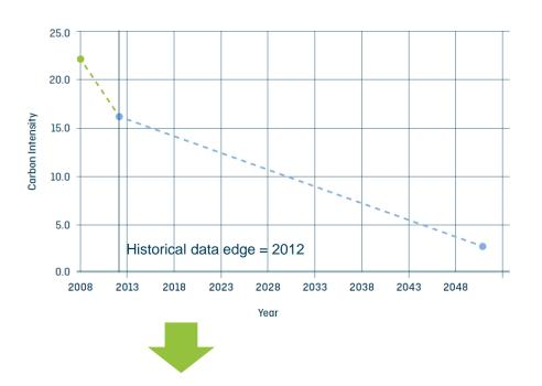
3. Transform into AER-equivalent trajectory by ship type & size (using 50% reduction target and 100 % reduction target)
